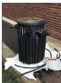
An old transformer in the basement of Baxter Hall was the culprit of the outage.
